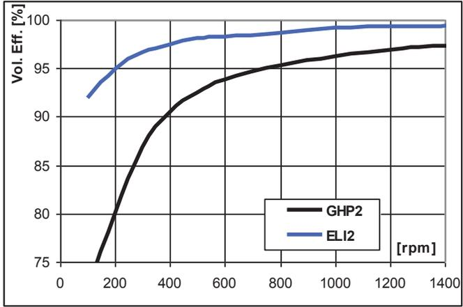
Comparison of volumetric efficiency at low rotation speed: Marzocchi GHP 2 – ELIKA ELI 2 , displacement 17.8 cm<sup>3</sup>/rev; P = 200 bar.
