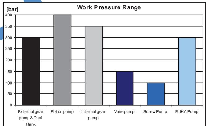
On side: comparison between the different fields of use of different kinds of volumetric pumps.
