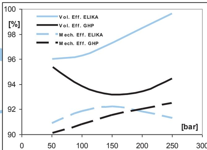
Efficiency pump comparison [%] Marzocchi GHP2 – ELIKA ELI 2, same displacement 17.8 cm<sup>3</sup>/rev.
