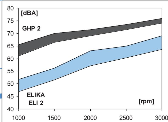
Noise pump comparison [dBA] Marzocchi GHP2 – ELIKA ELI 2, same displacement 17.8 cm<sup>3</sup>/rev.
