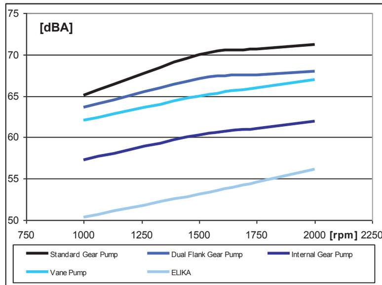
The low pulsation reduces the induced vibration in the machines. The lower frequency of the ELIKA pump produces a more pleasant sound. Pressure pulsation comparison between:
